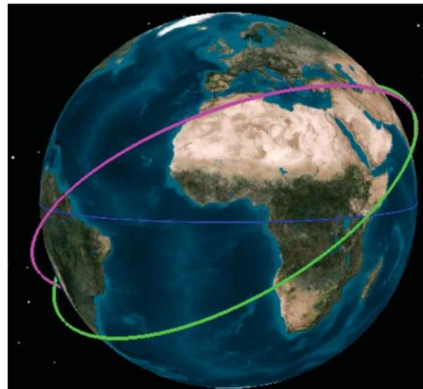
Fig. 8. Example of a configuration with the CYGNSS constellation (magenta) and 8 satellites in a plane at 35° (green). The coverage for different inclinations of the green plane are analyzed: 35°, 65°, 75°, and 85° (Satellite Tool Kit (STK) - Analytical Graphics, Inc (AGI))
