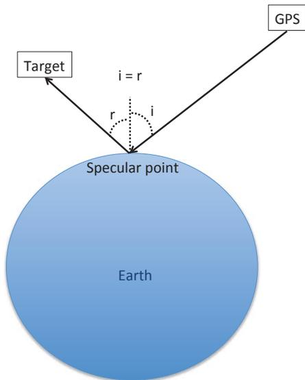
Fig. 1. Geometry of a specular point [11].
