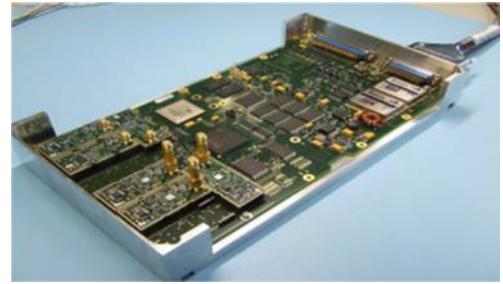
Fig. 2. SGR-ReSI SGR-ReSI, part of sea-state payload on TDS-1.
